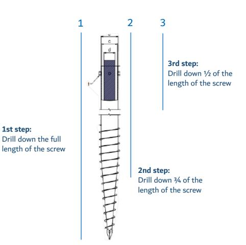
Must measure based on the diameter of screw without the threads to match depth. Vacuum hole to pull out debris every 6"
